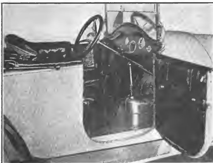
Control features of new Scripps-Booth, showing left drive and center gearshift as well as arrangement of instrument board
